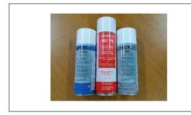
PT Chemicals <u>Visible Type</u> Penetrant: 907 PB Developer: NQI Cleaner: 9PR5
